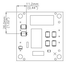
Figure 21: Temperature measurement location
