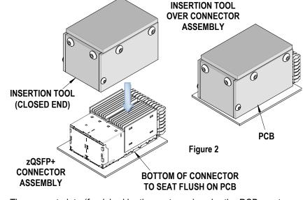
seat the connector assembly as shown. The support plate (furnished by the customer) under the PCB must have clearance for the connector pins as they pass through the PCB.
