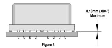
3. Using the application tool and an appropriate press, seat the vertical power module until there is less than 0.10mm (.004 in) clearance between the bottom of the plastic housing and the surface of the PCB. See Figure 3.
