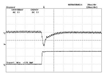
**Figure 20:** Typical transient response to step load change at 2.5A/μS from 50% to 100% of lo, max at 5Vin, 3.3Vout (Cout =1uF ceramic, 10μF tantalum)
