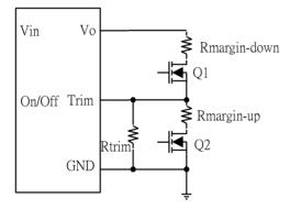
Figure 39: Circuit configuration for output voltage margining
