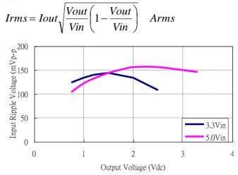
Figure 32: Input voltage ripple for various output models, Io = 6A (CIN = 2×100µF tantalum // 47µF ceramic)
