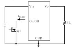
Figure 34: Positive remote On/Off implementation
