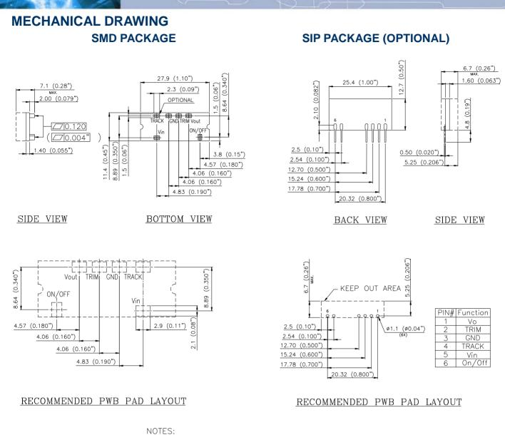
DIMENSIONS ARE IN MILLIMETERS AND (INCHES) TOLERANCES: X.Xmm±0.5mm(X.XX in.±0.02 in.) X.XXmm±0.25mm(X.XXX in.±0.010 in.)
