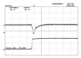
**Figure 22:** Typical transient response to step load change at 2.5A/µS from 50% to 100% of lo, max at 5Vin, 1.8Vout (Cout = 1uF ceramic, 10µF tantalum)
