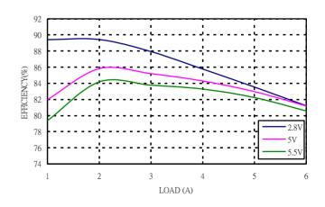
Figure 6: Converter efficiency vs. output current (0.75V out)
